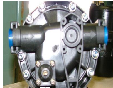
Pressure adjust on pump
