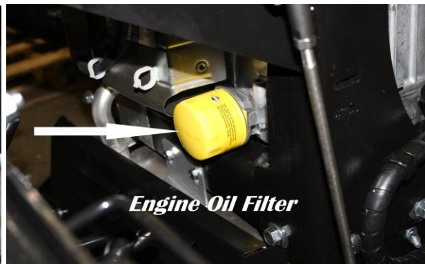
(remove oil filter and replace with new)
