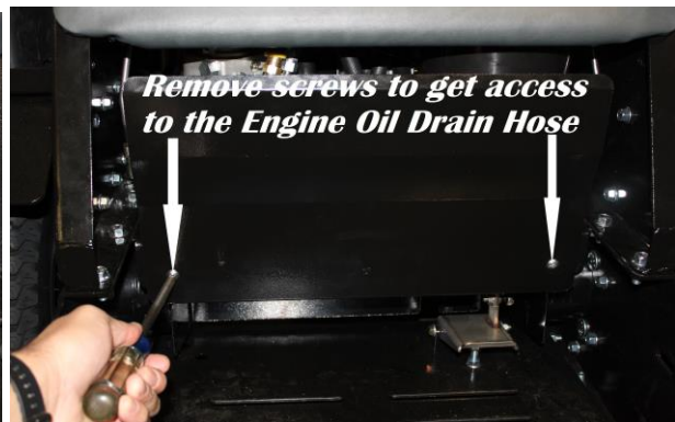
(remove Hydro Shield to access drain hose)
