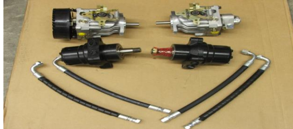
(hydraulic motors, pumps and hoses)
