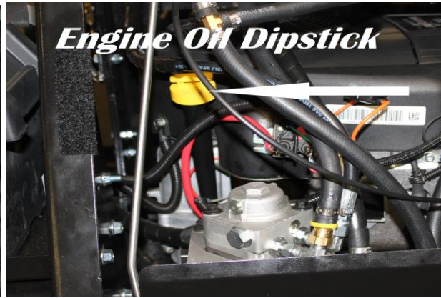
(Fill oil and check for proper fill level)
