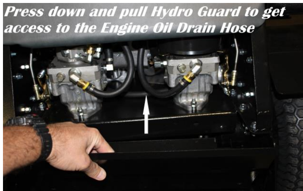
(remove Hydro Shield for easier access)
