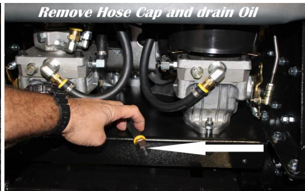
(pull drain hose out from between hydro's)
