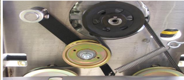
(idler bracket, idler pulley and drive belt)
